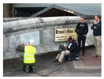
Plate-thickness measurements have been carried out by our volunteer friends from the British Institute of Non-Destructive Testing using Ultra-Sonic test equipment. Subsequent tests using sophisticated Pulsed Eddy Current equipment were carried out courtesy of Baugh & Weedon.
